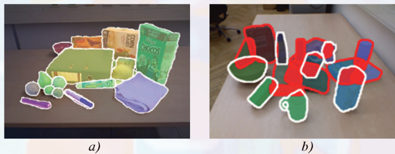
Fig. 3. Unknown objects segmentation: a – segmentation without taking into account overlapping parts of objects [21]; b – amodal instance segmentation [23]
