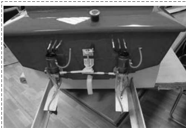
Fig. 7. Propulsion and steering complex of the boat
