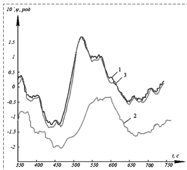
Fig. 2. Deviation angles of GSP, where 1 — deviation angles of GSP of the real system; 2 — estimations of the GPS deviation angle using adaptive Kalman filter [3]; 3 — deviation angle of GPS with correction from AAS in the output signal
